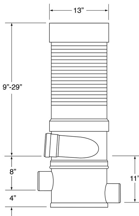
**VORTEX-150:** The Vortex-150 filter body consists of an upper section with a rainwater inlet, a middle section with a clean water outlet, and a lower section with a waste outlet. All three sections can be rotated independently. The inlet is a 150mm gasketed socket that accepts 6" SDR pipe; the clean water outlet is a 100mm spigot that can be connected to a 4" pipe using a 4" flexible coupling, and the waste outlet is a 150mm spigot that can be connected to 6" pipe using a 6" flexible coupling.
